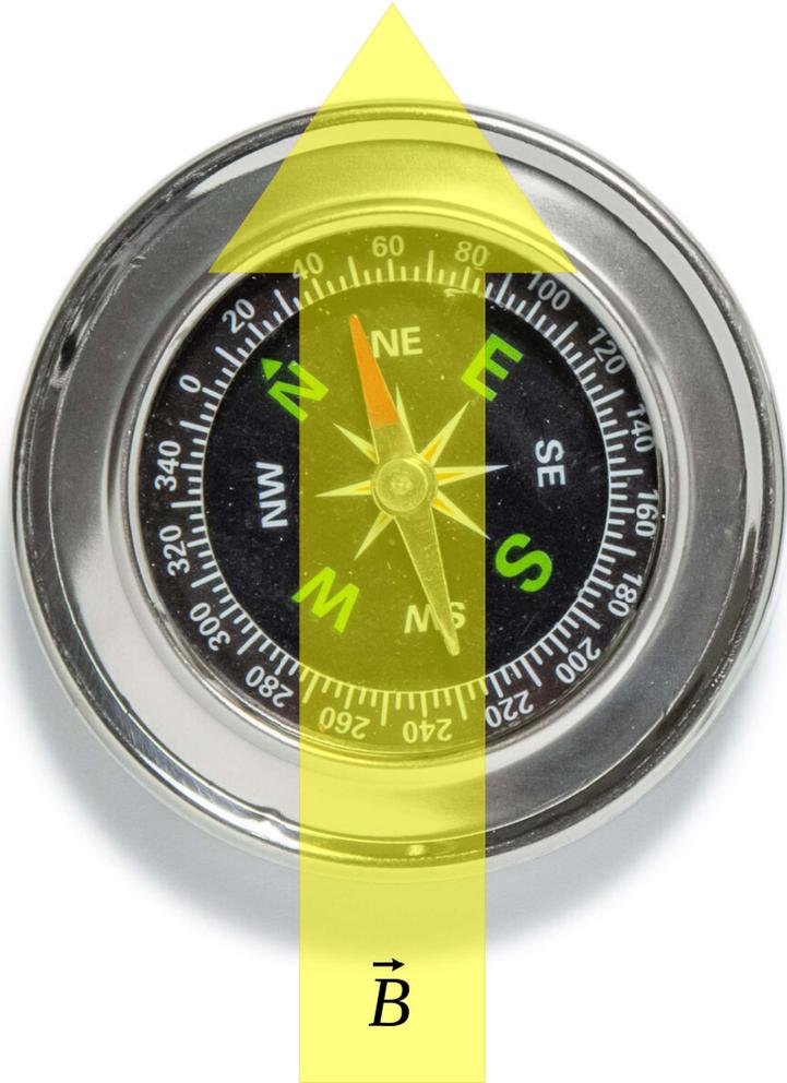
$$\begin{aligned}\vec{T} &= \vec{M} \times \vec{B} \\ \vec{L} &= \gamma \vec{M} \\ \frac{d\vec{M}}{dt} &= \vec{T} = \gamma \vec{M} \times \vec{B}\end{aligned}$$
