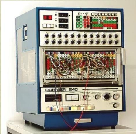
Analogous computational machine (ACM) is a physical system, which models its own dynamics
