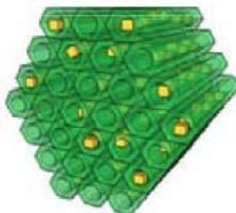
Nanoparticles in Mesoporous Silica (SBA-15)
